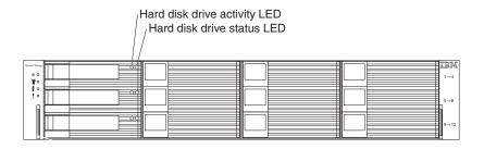
Figure 45. Hard disk drive LEDs
